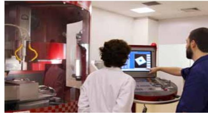
The X-Ray Computer Tomography allows the analysis of the internal and external structure of assembled parts as well as of homogeneous components.
