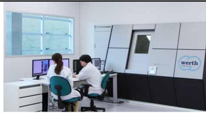
The X-Ray Computer Tomography allows the analysis of the internal and external structure of assembled parts as well as of homogeneous components.
